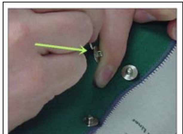
Figure 5. Glue the snap to the liner using SuperGlue
